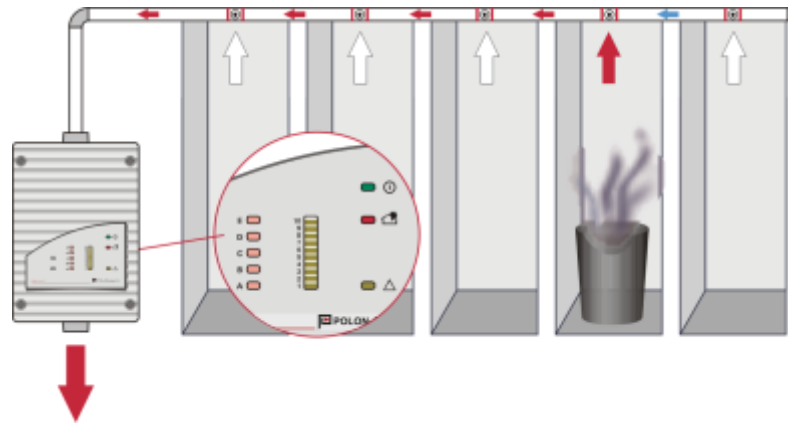
Image 6: Phase 2 ROOM IDENT Very early fire detection.
