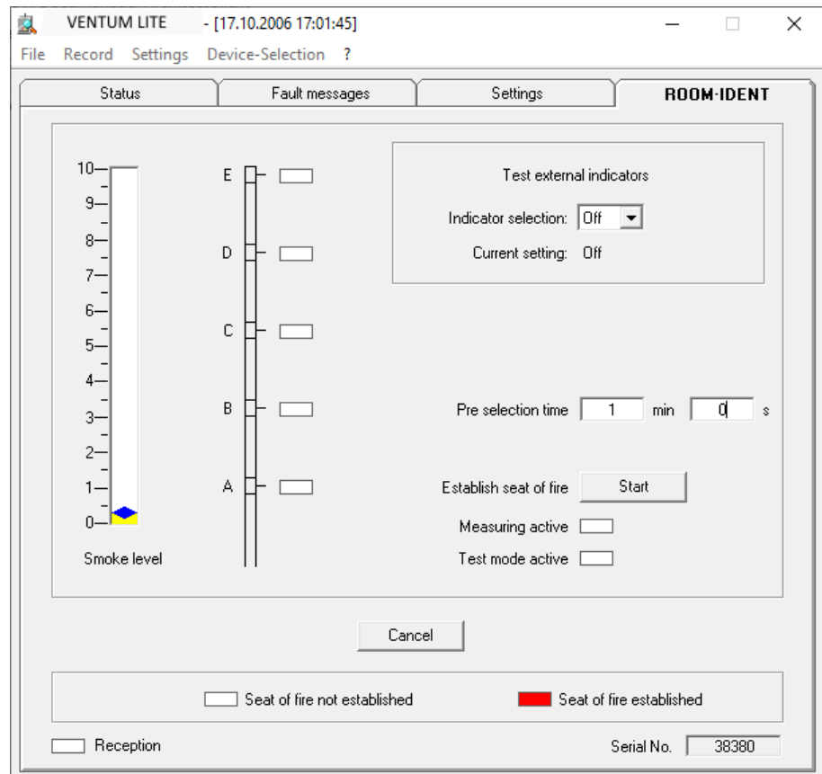
Image 145: Checking ROOM-IDENT and response indicators
