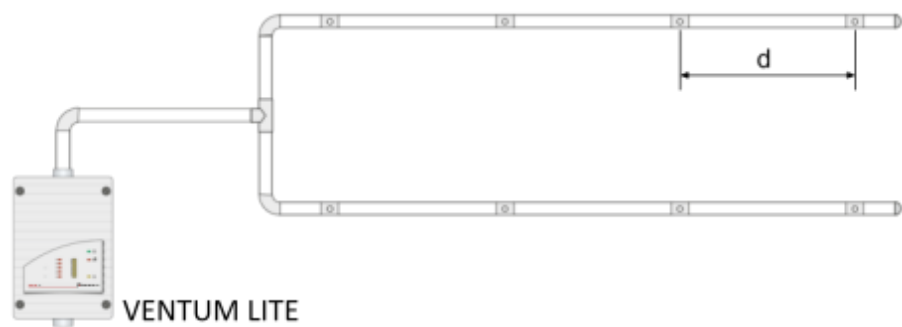
Image 53: U-pipe system, e.g. for equipment monitoring
