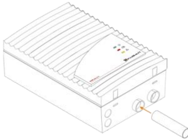
Image 112: Installation of the aspiration pipe
