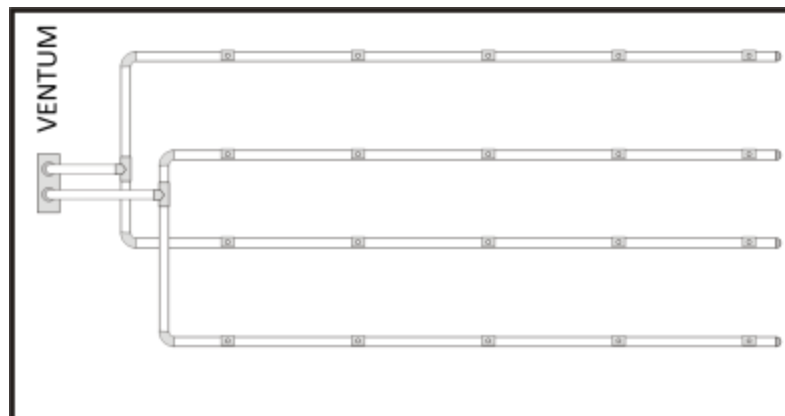
Image 39: Example pipe configuration with dual detection dependency
