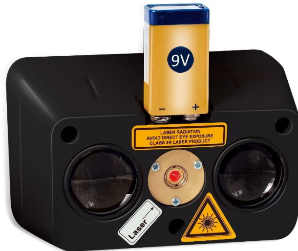
Fig. 5.1. DOP-3000 detector during optical path alignment
