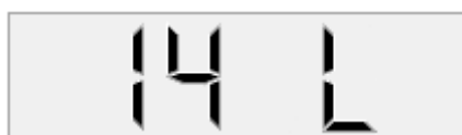
Fig. 4.2.5.1 The control panel screen when a magnet is close to detector number 14.
