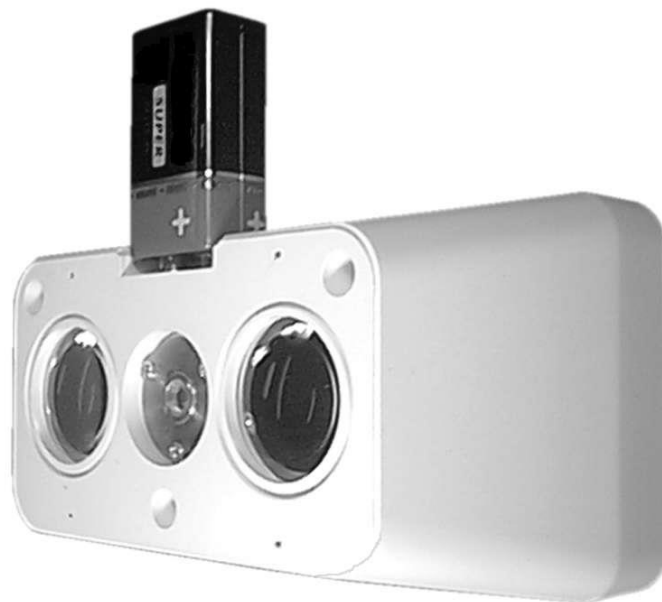
Fig. 2 DOP-6001R detector during optical path alignment
