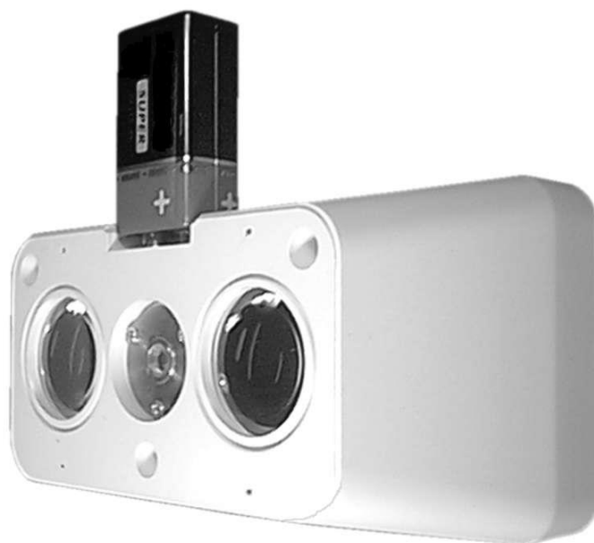
Fig. 2 DOP-6001 detector during optical path alignment
