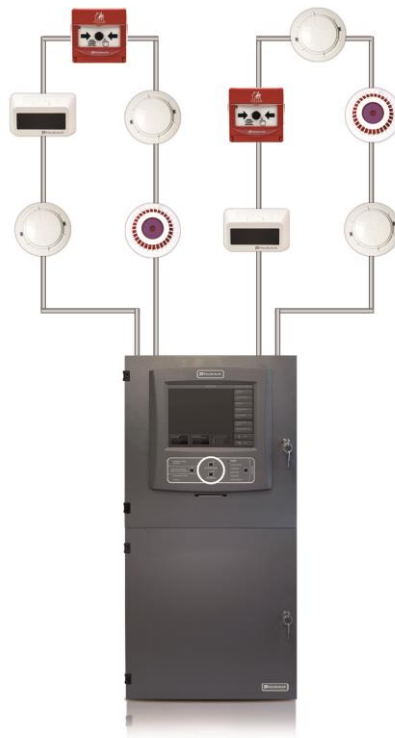
Figure 2.2/1 Example configuration of POLON 6000 with non-distributed (traditional) architecture
