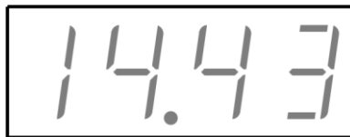
Figure 8.1. Example of the time displayed on the LED screen when no fault occurred.
