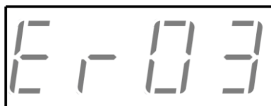
Figure 8.2. Example of fault number 3 displaying
